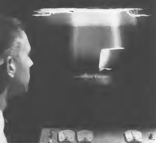
Melting columbite and tantalum in the 6000-deg. F interior of an electron beam furnace—a part of the advanced metals technology produced at Haynes Stellite. These metals and others—produced by the latest techniques—give you the tools to solve problems even at temperatures of 2300 deg. F and higher.
